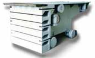
Compaction trolley with rolls to reduce friction and wearing
